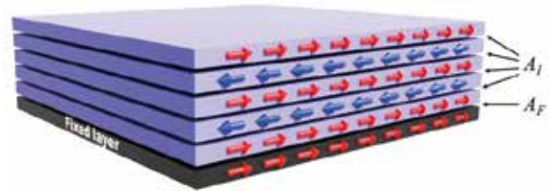
Fig. 1 Schematic representation of a 5-layer SAF for bimerons stabilization with one fixed layer.
