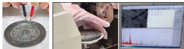
Fig. 2 (Left) Electrical conductivity test of a bronze mirror. (Right) SEM-EDS analysis of a small bronze mirror in the Comprehensive Bronze Mirror Project at IMR.
