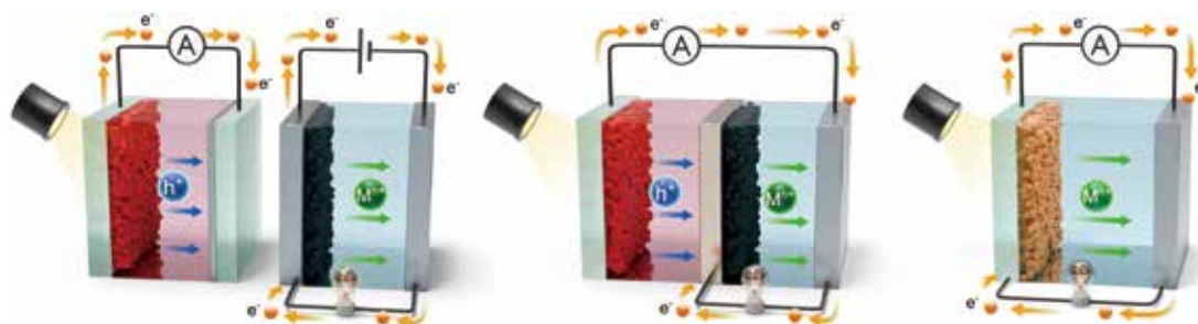
Fig. 1 Schematic illustration showing the fundamental structures for the separated system (left), as well as the integrated three-electrode (middle) and two-electrode (right) photobatteries [1].
