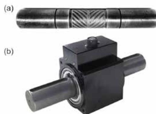
Fig. 1 (a) The shaft for rotating-torque sensor with thermal-spraying film of (Fe, Co) 72 Si 4 B 20 Nb 4 amorphous alloy, and (b) the developed product of the rotating-torque sensor.
