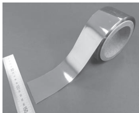
Fig. 1 Outer appearance of a 50 mm-width ribbon fabricated by melt-spun technology [2].
