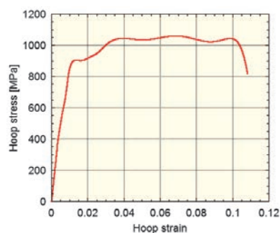
Fig. 2 Hoop stress and hoop strain curves in Cu inner pellets with 1 and 2 mm specimen width.
