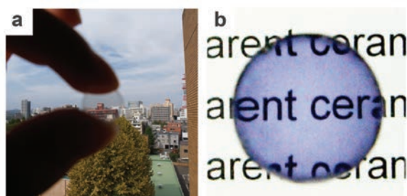
Fig. 1 (a) \text{Lu}_2\text{O}_3 and (b) \text{Nd}^{3+} -doped \text{Lu}_2\text{O}_3 transparent polycrystalline ceramics produced by spark plasma sintering. The diameter of the ceramics is 10 mm.
