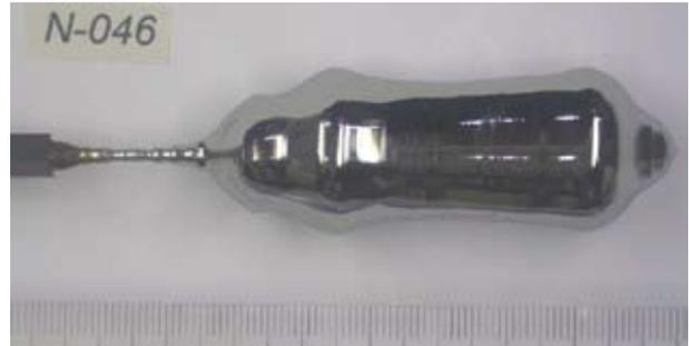
Fig. 2 A photograph of a Ge single crystal grown from  $B_2O_3$ -partially-covered Ge melt.
