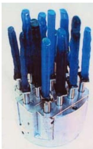
Fig. 1 Assembled single crystals of the spin-Peierls compound CuGeO<sub>3</sub>.
