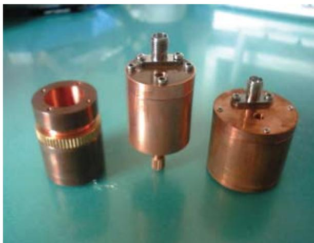
Fig. 1 A cylindrical cavity with the resonant frequency around 6.3 GHz used for the cavity perturbation technique to evaluate the intrinsic magneto-resistance of carbon nanotube. The sample is located at the position where the microwave electric field is along the SWNT.
