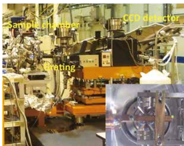
図2:超高分解能X線発光分光器とチャンバー内のミニチュアマグネット Figure 2: Resonant Inelastic X-ray Scattering with Ultrahigh Resolution Soft X-ray Emission Spectrometer and Miniature Magnet in the Sample Chamber
