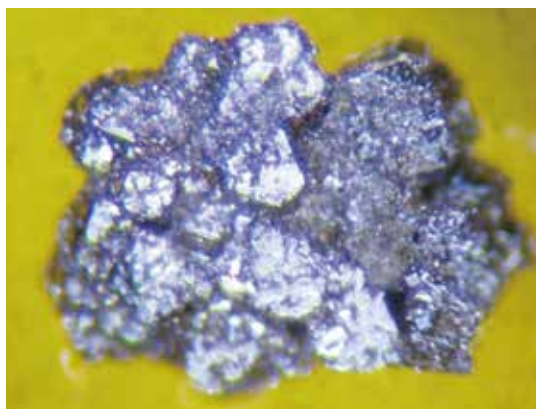
図1: ネプツニウム化合物で初めての超伝導体 \text{NpPd}_5\text{Al}_2 Figure 1: First neptunium-based superconductor \text{NpPd}_5\text{Al}_2
