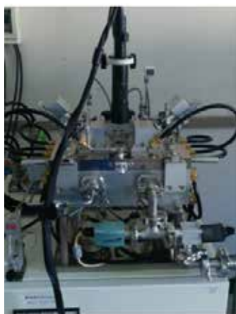
図1: その場観察装置とSi多結晶の固液界面不安定化の様子 Figure 1: In situ observation system and images of Si crystal/melt interface
