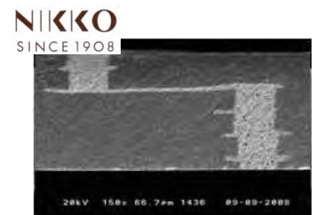
LTCC with electrical feedthrough for MEMS packaging (Nikko)
