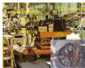
超高分解能軟X線発光分光器とチャンバー内のミニチュアマグネット Resonant Inelastic X-ray Scattering with Ultrahigh Resolution Soft X-ray Emission Spectrometer (Miniature Magnet in the Sample Chamber)
