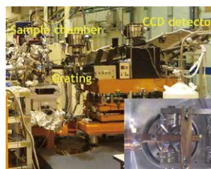
超高分解能X線分光器とチャンバー内のミニチュアマグネット Resonant Inelastic X-ray Scattering with Ultrahigh Resolution Soft X-ray Emission Spectrometer (Miniature Magnet in the Sample Chamber)
