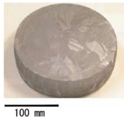
Fig.2 Outlook of an extremely high-quality Si multicrystal ingot with the same grain orientation and large grain size grown by the dendritic casting method.
