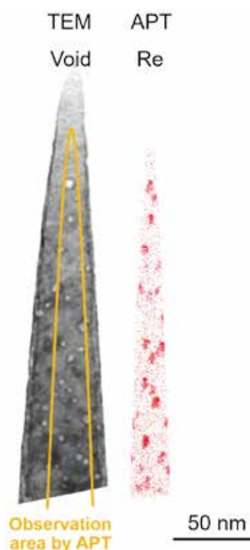
Fig. 1 TEM image and APT map for Re obtained from the same needle specimen of (initially pure) W neutron-irradiated in the fast-neutron experimental reactor Joyo. A one-to-one correspondence was clearly obtained between the voids in the TEM image and the Re-enriched clusters in the APT map.
