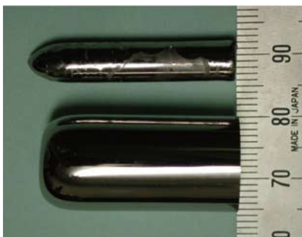
Fig. 1 Outer appearance of the W.Q. Ni 60 Pd 20 P 20 (d = 6 mm) and W.Q. Ni 60 Pd 20 P 17 B 3 (d = 15 mm) bulk samples.
