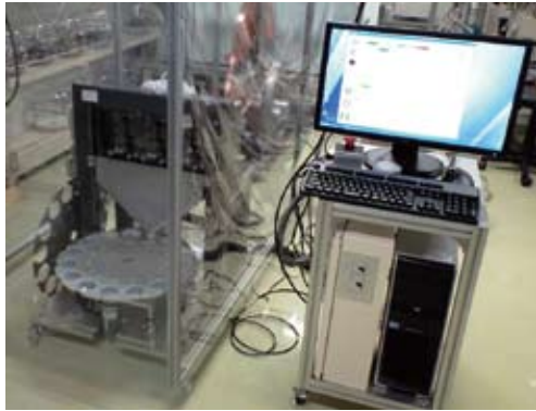
Fig. 1 Outer appearance of automatic weighing machine, right: computer and controller board, left; shearing and weighing machines with turn table for 15 samples, back; materials feeder of three metals, Cu, Ni and Al.
