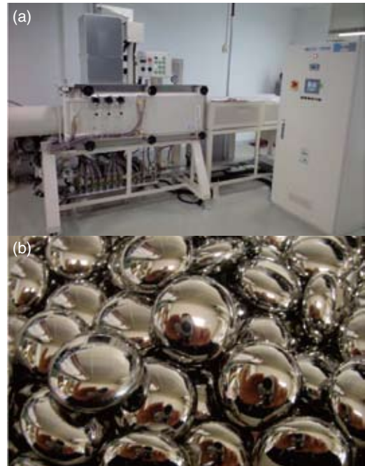
Fig. 2 Outer appearance of automatic master alloy fabrication machine (a)[1], photo of fabricated Zr_{55}Cu_{30}Ni_5Al_{10} master alloys using the automatic master alloy fabrication machine (b).
