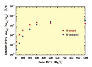
Fig. 2 Dose rate dependence of  $\Delta RIC$  ( $\Delta RIC = \sigma_{RIC} - \sigma_{BC}$ ).
