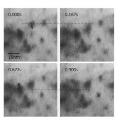
Fig. 2 In-situ observation of 1D motion of SIA clusters in A533B under electron irradiation at room temperature.
