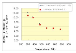
Fig. 3 comparison of thermal diffusivity data of irradiated Hf hydride disk with un-irradiated one
