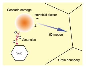
Fig. 1 'Production bias mechanism' for void swelling under cascade damage condition.
