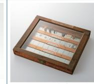
Corrosion resistance test samples of Cr-Mo steel
